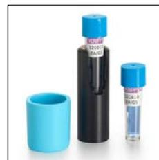
5. Take a Verify indicator that has not been autoclaved and label it as the positive control. Activate this indicator as described above.
