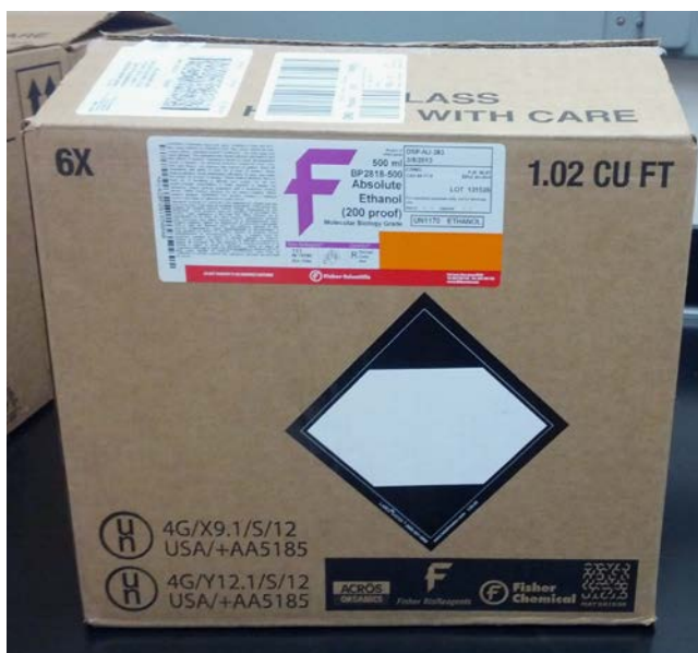
Figure 2. DOT specification packaging with square on point label
